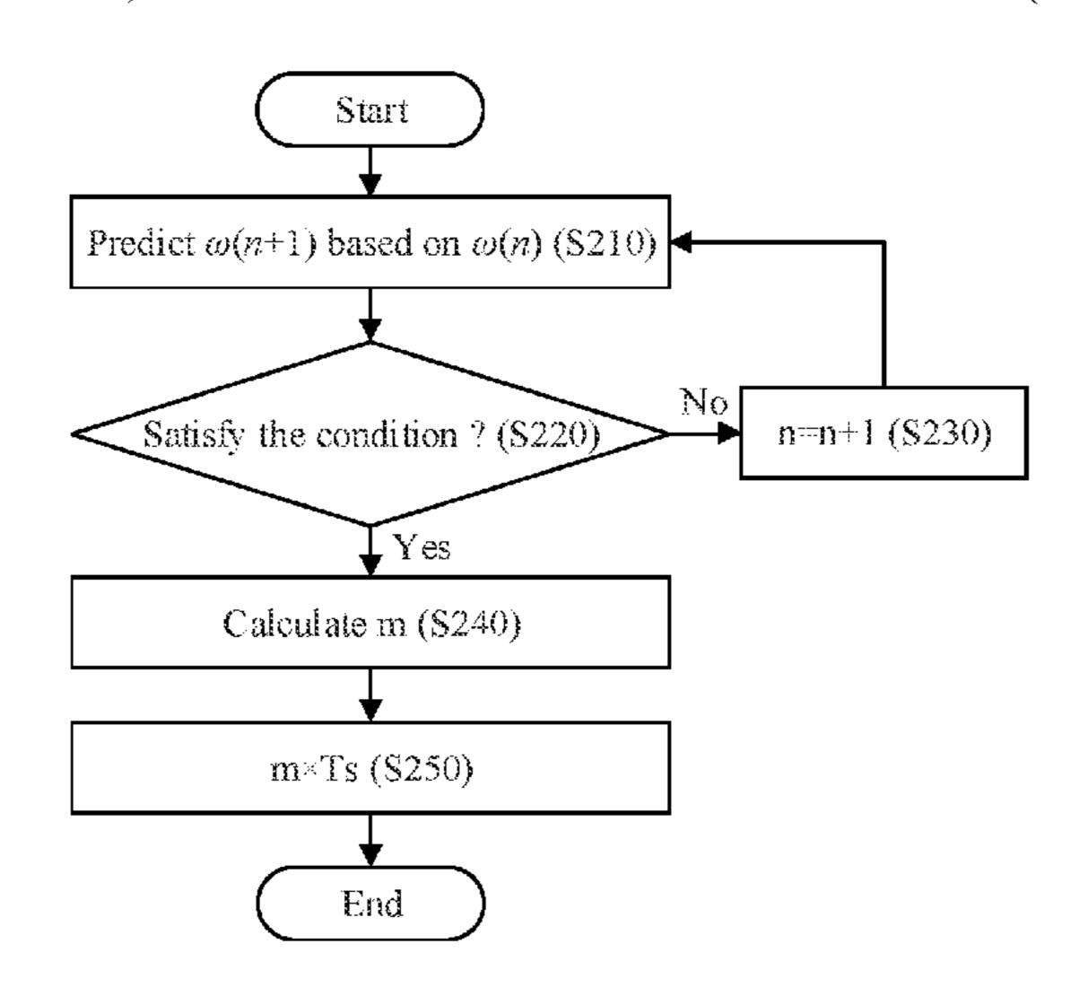
without affecting a recovery of the wind turbine after the primary frequency modulation; controlling the output power based on the determined frequency modulation remaining time.
