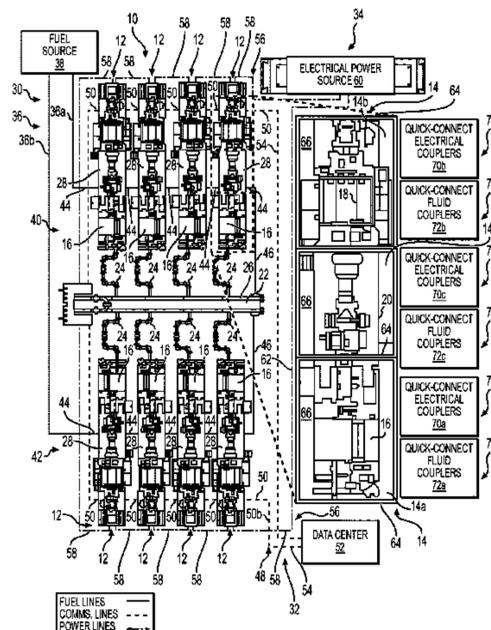
positioned to receive respective electrical and fluid connections of the component electrical and fluid assemblies and connect to other portions of the hydraulic fracturing unit.
