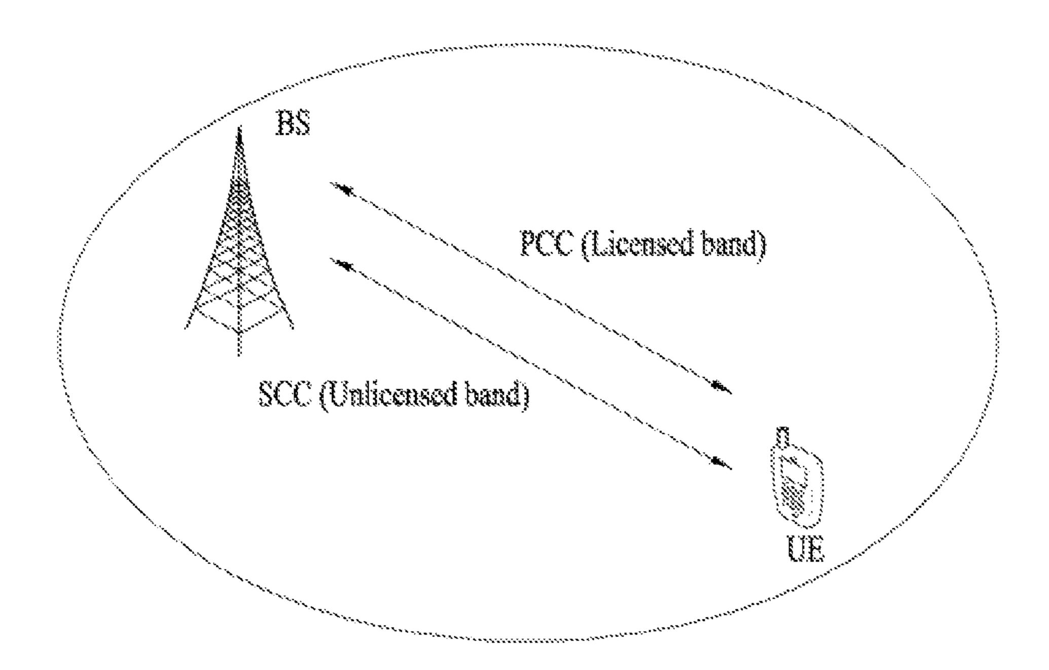
Carrier aggregation between L-band and U-band
