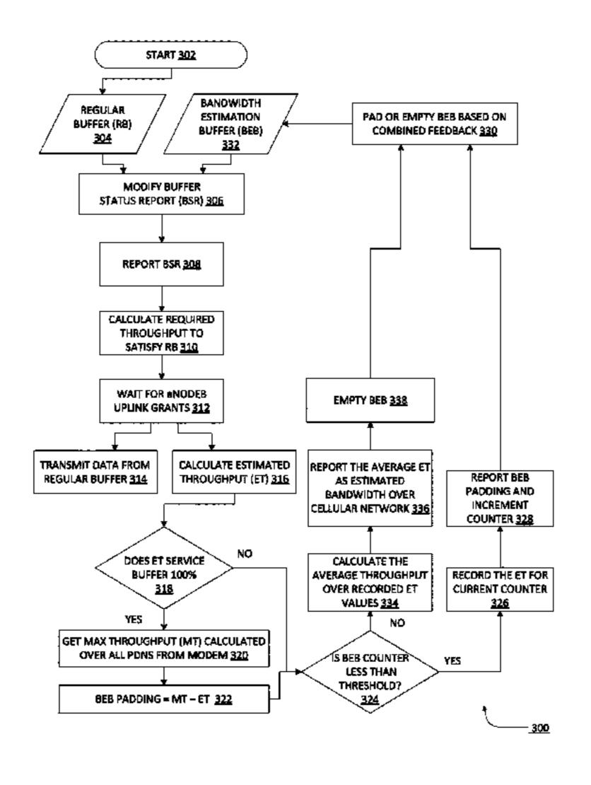
calculating estimated throughput from the user equipment, determining if the estimated throughput services the data amount stored at the regular buffer and in response to the estimated throughput being insufficient to service the data amount stored the regular buffer, determining if a counter is less than a threshold value.
