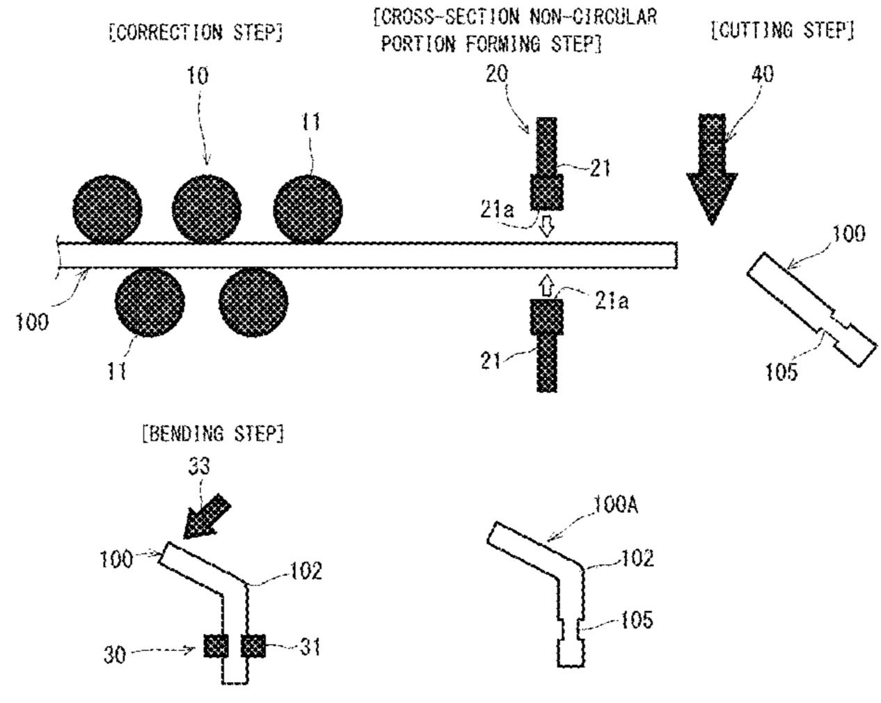
section non-circular portion causes relative rotation between the cross-section non-circular portion and the wire holding portion to be suppressed as compared with a case of the cross-section circular shape. Accordingly, bending accuracy in the three-dimensional shape for the round metallic wire is improved.
