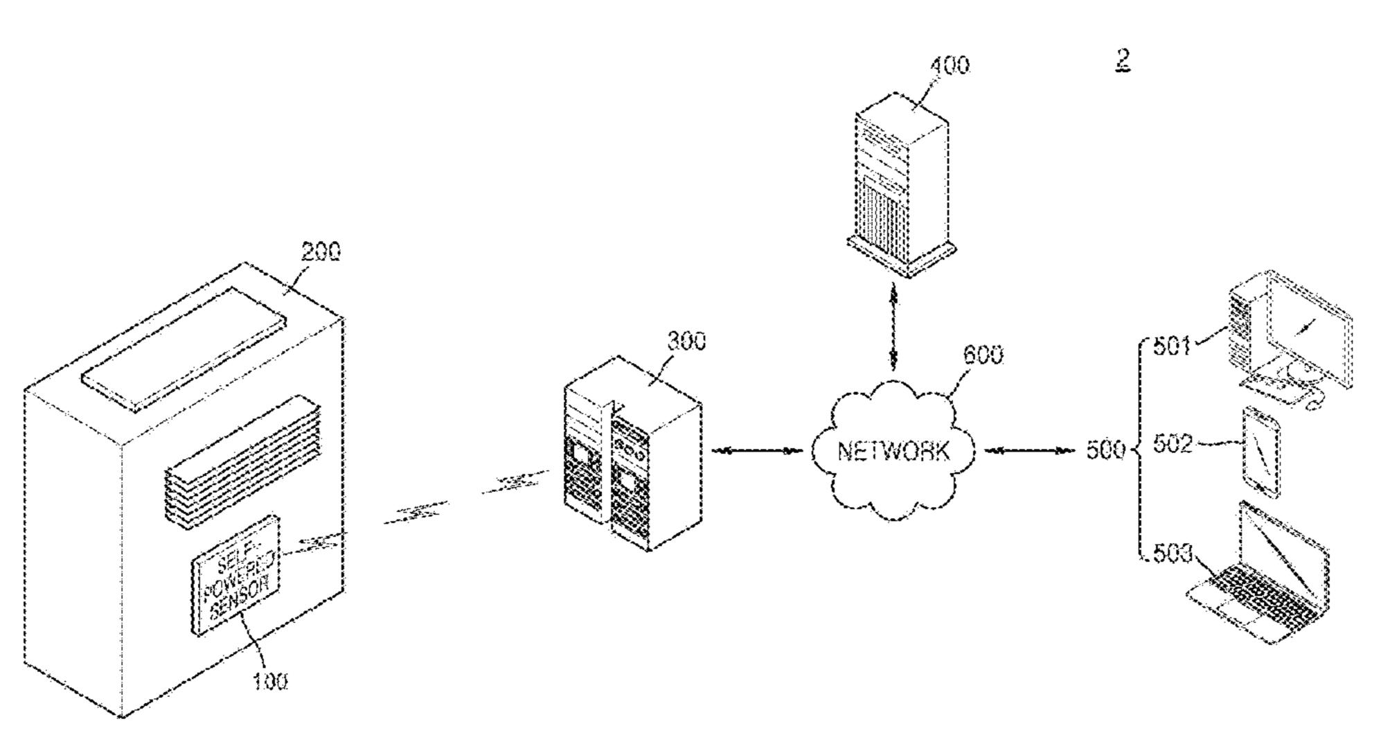
storage amount of the electrical energy stored in the electrical energy storage unit and a reference storage amount. The sensing unit may also include a processor generating and wirelessly transmitting a sensing signal based on the electrical energy stored in the electrical energy storage unit when the switching unit switches to the energized state.
