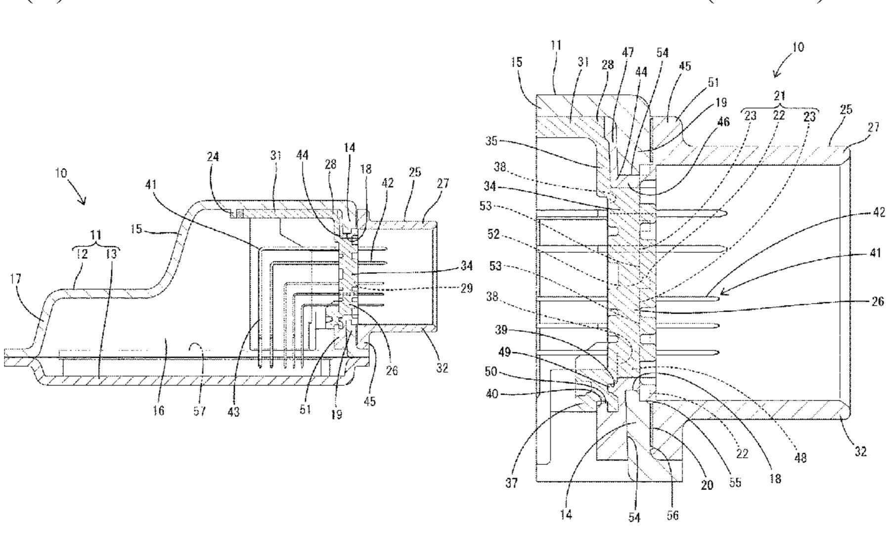
contact with at least one of an outer surface and an inner surface of the protruding portion. Since the inclination restricting portion is in contact with the protruding portion, the inclination of the terminal holding member with respect to the case is suppressed even if the terminal holding member is subjected to vibration.
