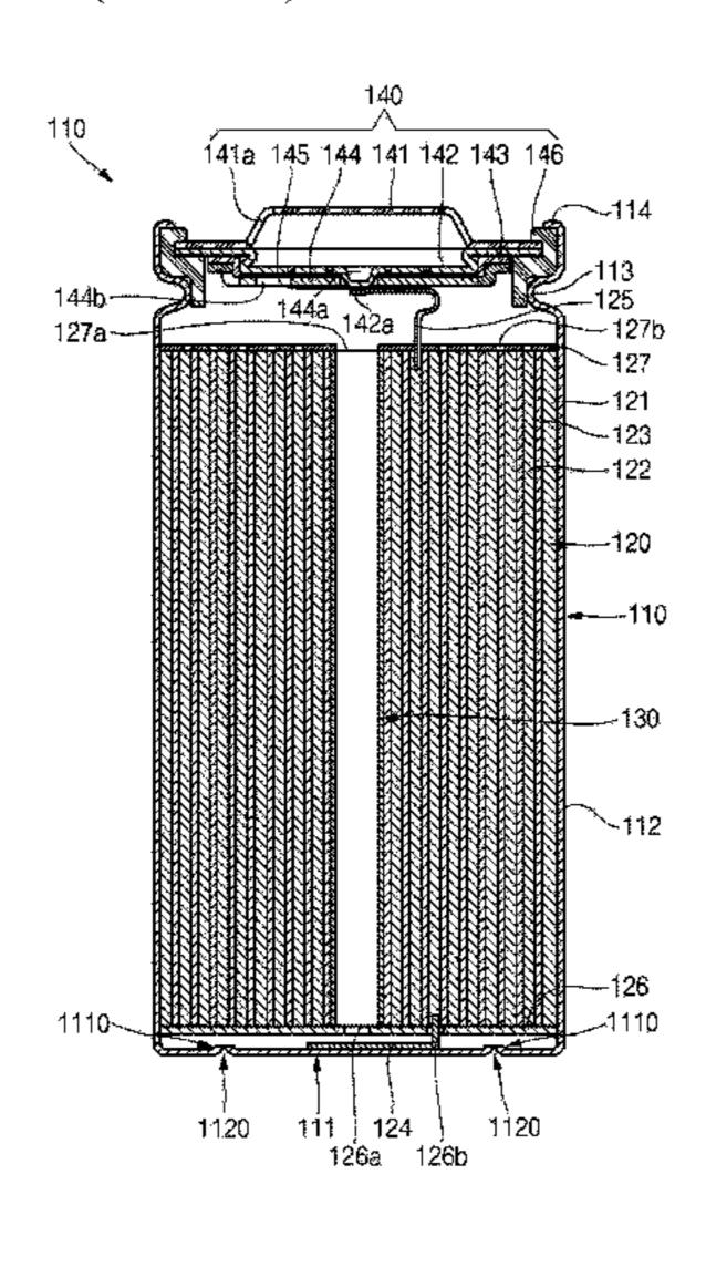
the cylindrical can, wherein the cylindrical can comprises a circular floor portion, a curved portion curved from the floor portion towards the electrode assembly, and a safety vent formed on the curved portion.
