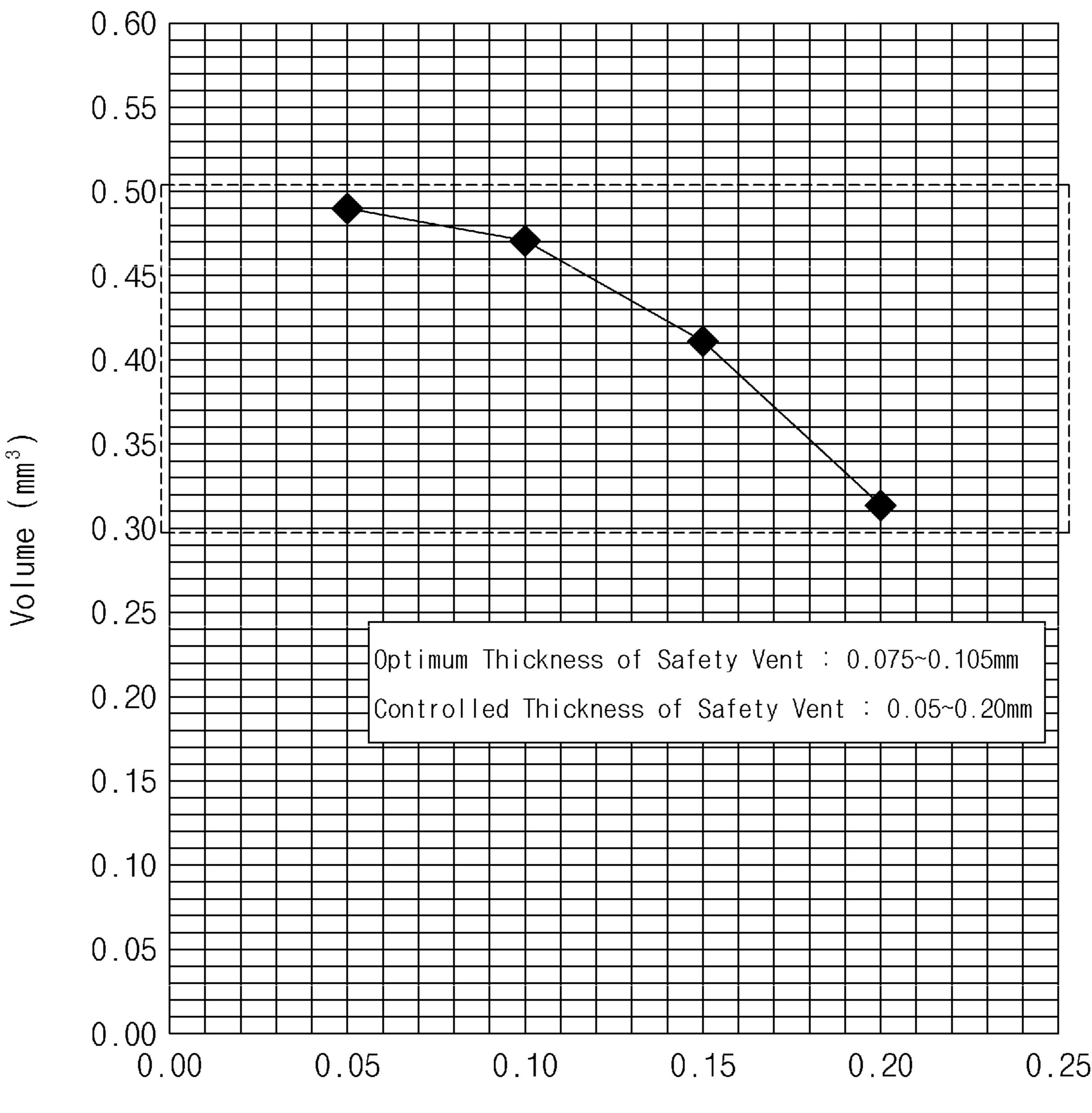
Thickness of Safety Vent (mm)
