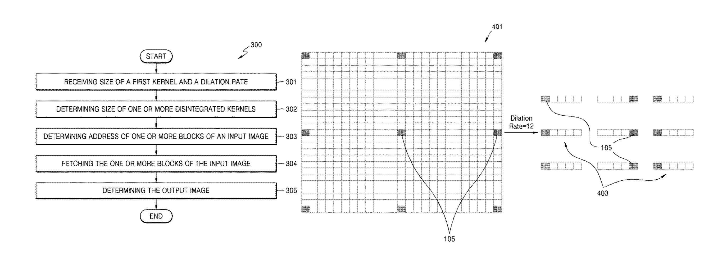
output image is obtained based on convolution of each of the one or more disintegrated kernels and the one or more blocks of the input image.
