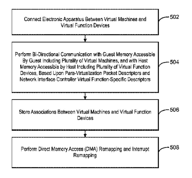
communicatively coupled to the descriptor hub and to store associations between the virtual machines and the virtual function devices. The electronic apparatus further includes an input-output memory map unit (IOMMU) to perform direct memory access (DMA) remapping and interrupt remapping.
