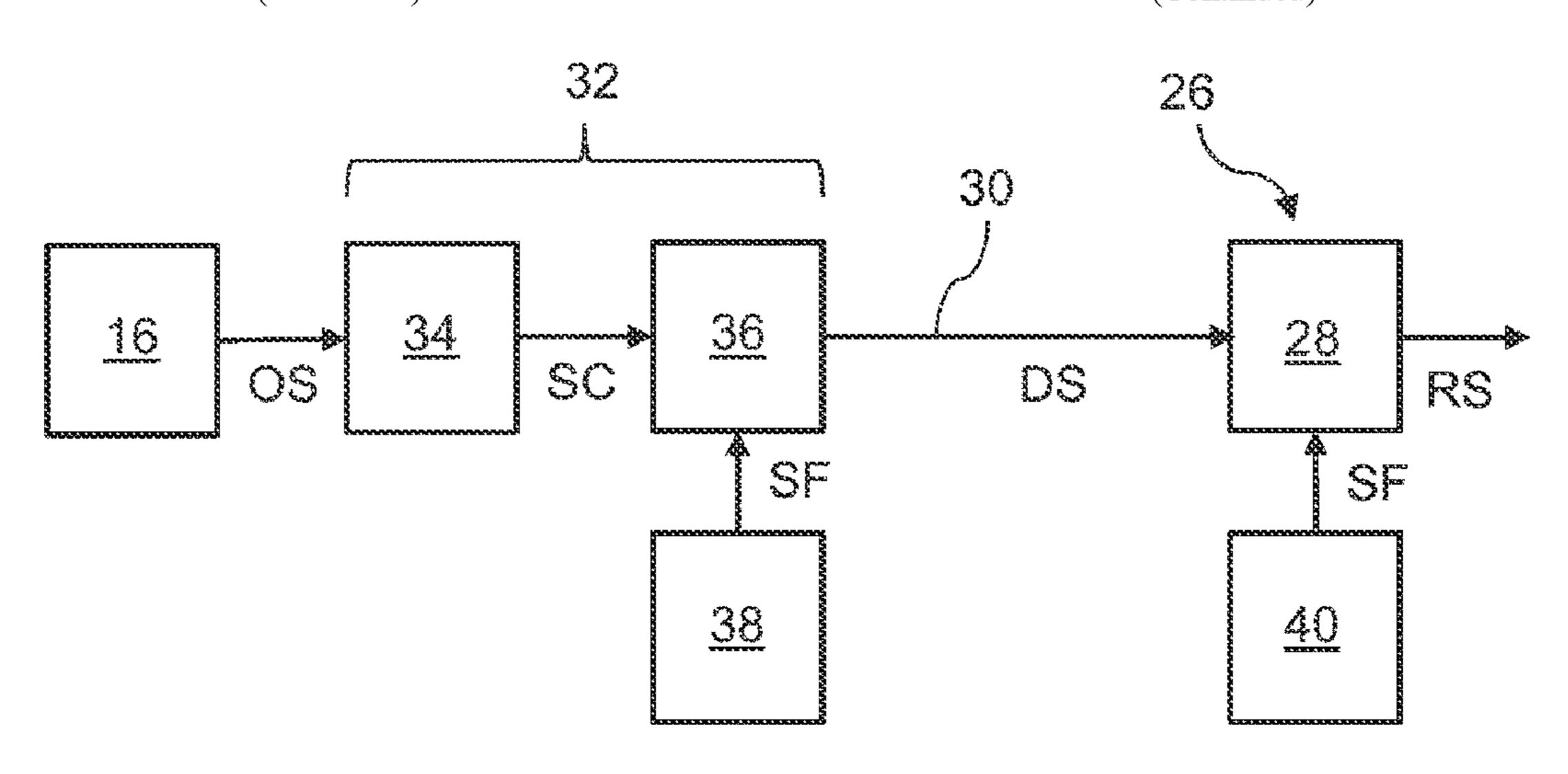
signal receiver (28), and (iii) outputting the scaled signal change (SC) as the digital sensor signal (DS). A corresponding apparatus (32) is disclosed for creating a digital sensor signal (DS) from an ultrasonic sensor (16) for signal transmission to a signal receiver (28), to a corresponding ultrasonic sensor device with an ultrasonic sensor (16) and such an apparatus (32), and to a corresponding ultrasonic sensor system (14).
