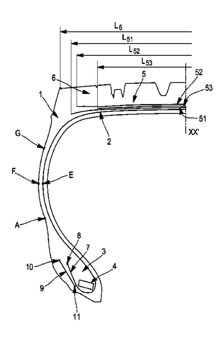
being present within the cords, and, in the sidewall of the tire, the profile of the outer surface of the tire is at a constant distance from the carcass reinforcement layer between the points F and A, and meets the outer surface of the bead at the point C, forming two successive circular arcs.
