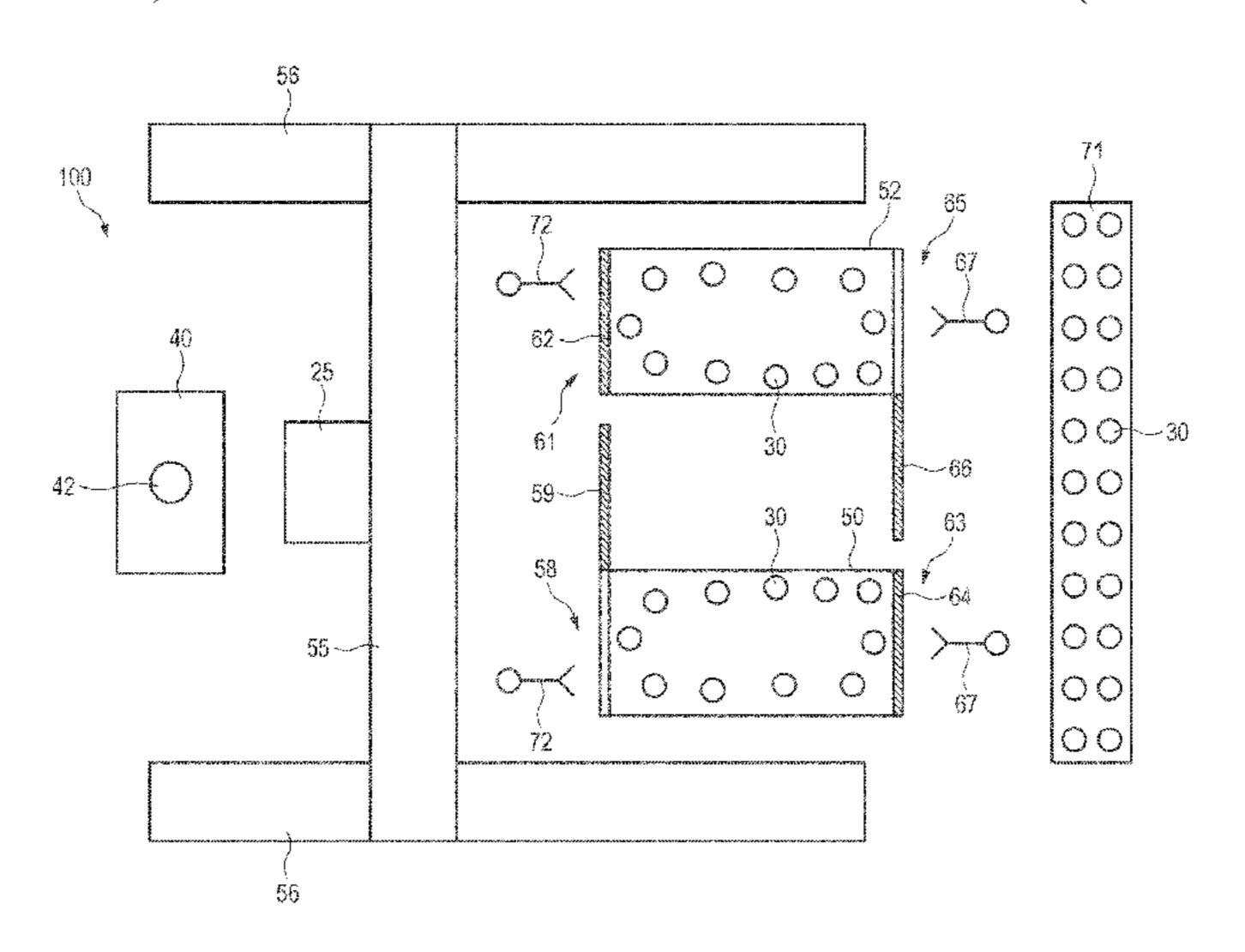
tool magazine is active at a time, so that exclusively the tool set from the respective active tool magazine is used for machining the clamped workpiece. There is also provided a corresponding method of machining workpieces.
