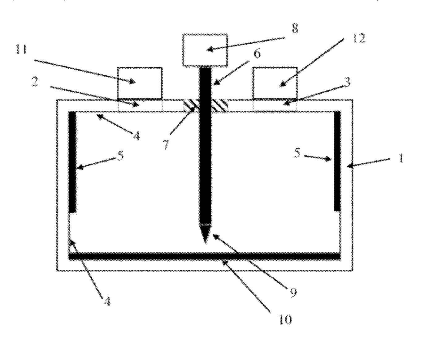
entirely or partially and is grounded. An electrode protrudes into the reactor, and this electrode is isolated from the grounded surface. High-voltage pulses are supplied to the electrode. The pulses cause formation of corona discharge streamers in a gap between the electrode and the conductive surface of the reactor.
