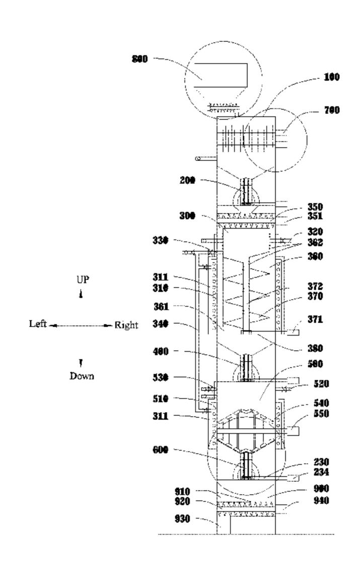
material is transported to a cracking unit for preheating, then heated and cracked under an inert atmosphere or vacuum to obtain cracked gas, solid cracked products and non-crackable products; and the solid cracked products and the non-crackable products are transported to a pyrolysis unit for pyrolysis at an aerobic atmosphere to obtain pyrolysis gas and non-pyrolysis products.
