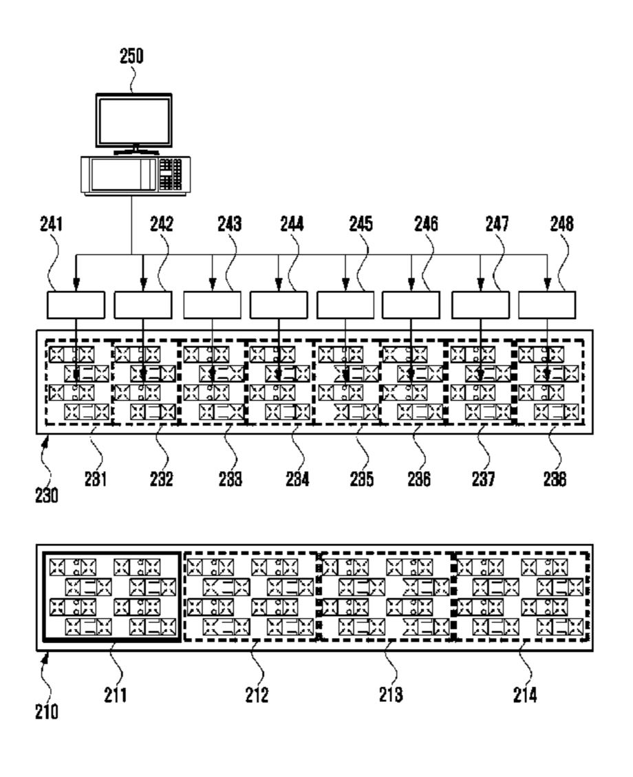
controlling the second antenna module by grouping each antenna element of the second antenna module into at least one antenna element group.
