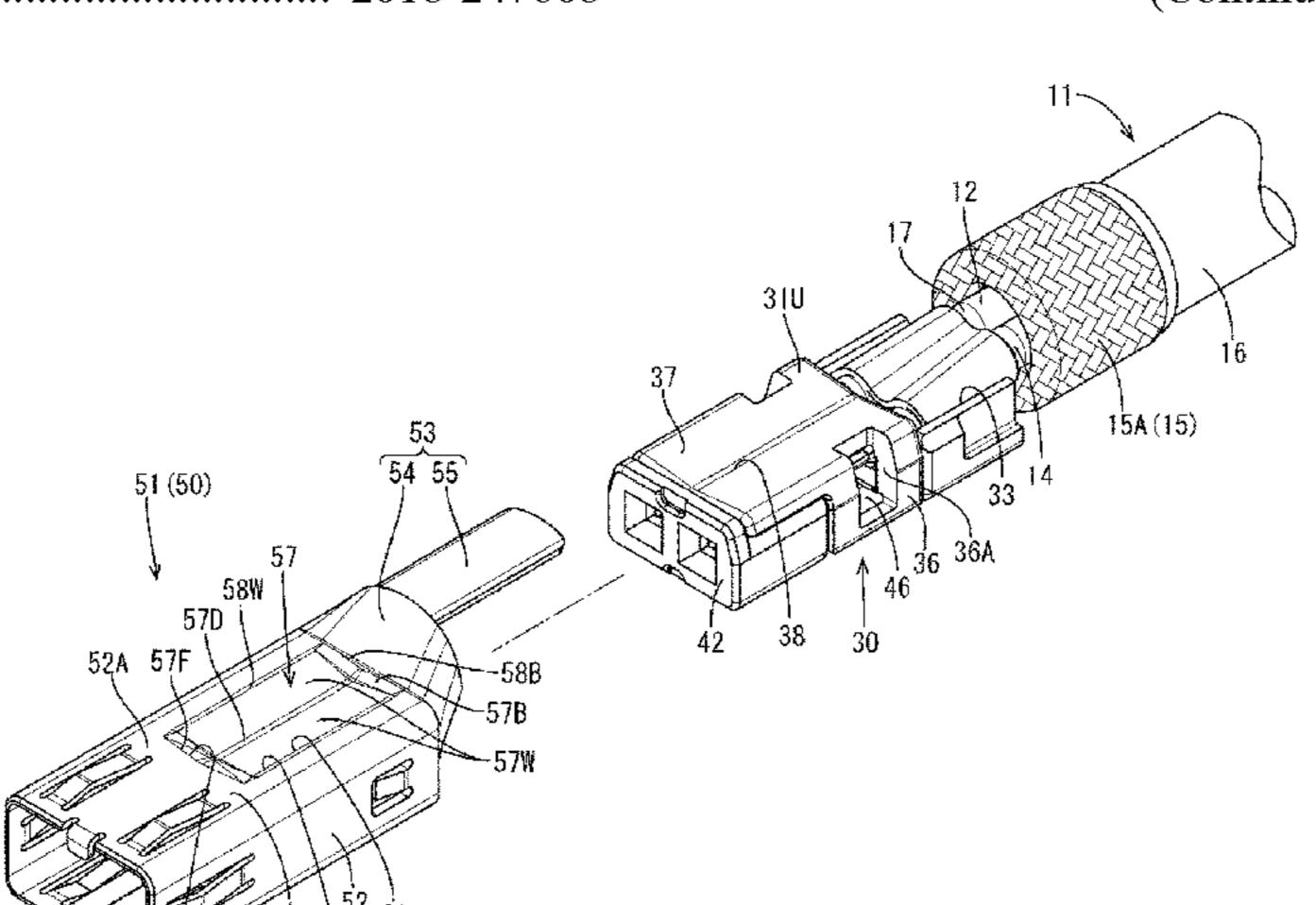
circumferential direction. The tubular portion 52 includes a depressed portion 57 arranged inside to radially face the fixing barrels 62 and allowing the fixing barrels 62 to be crimped by causing the fixing barrels 62 to be excessively deformed beyond proper crimping positions.
