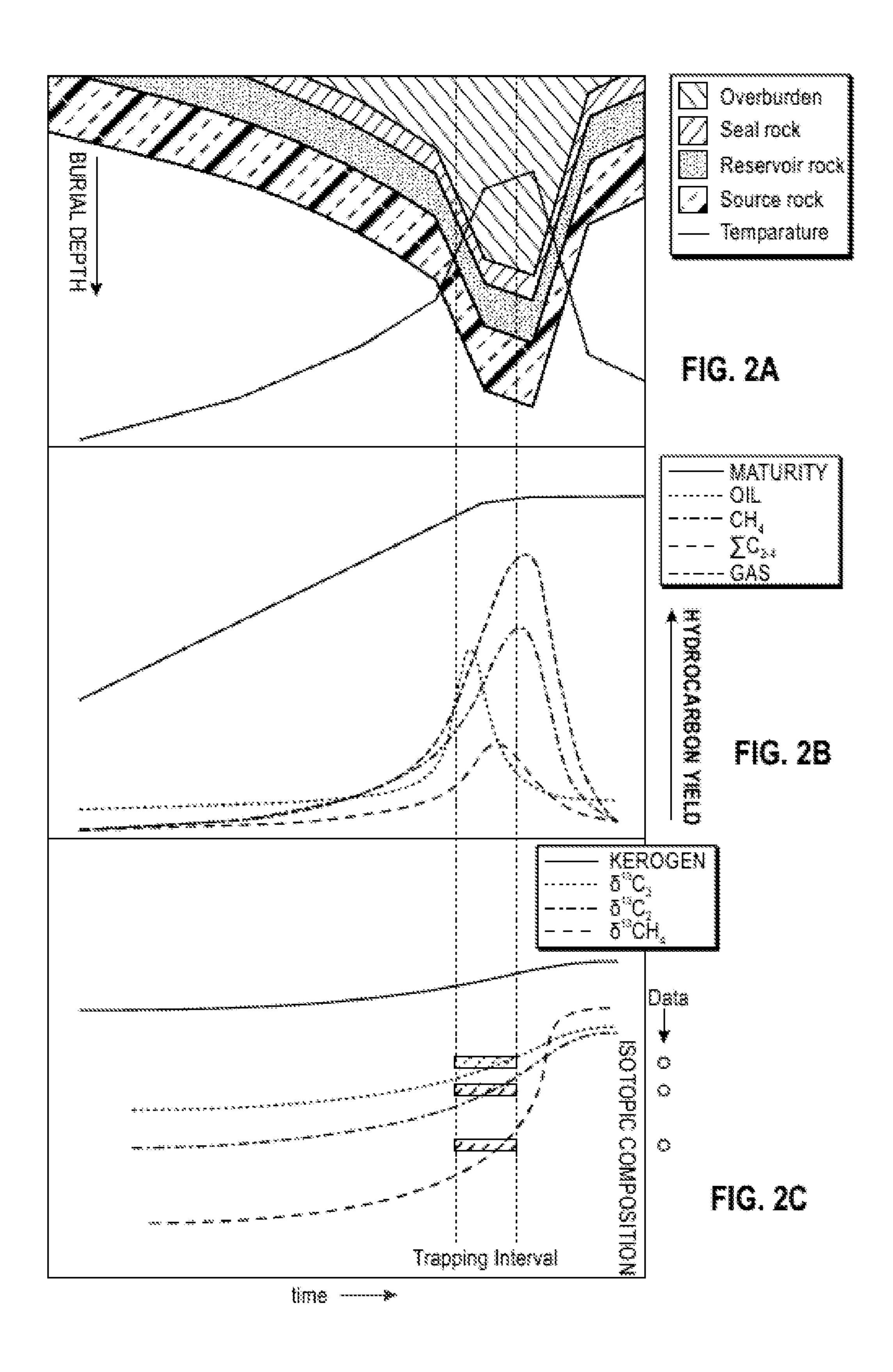
Cascading Cracking Scheme
