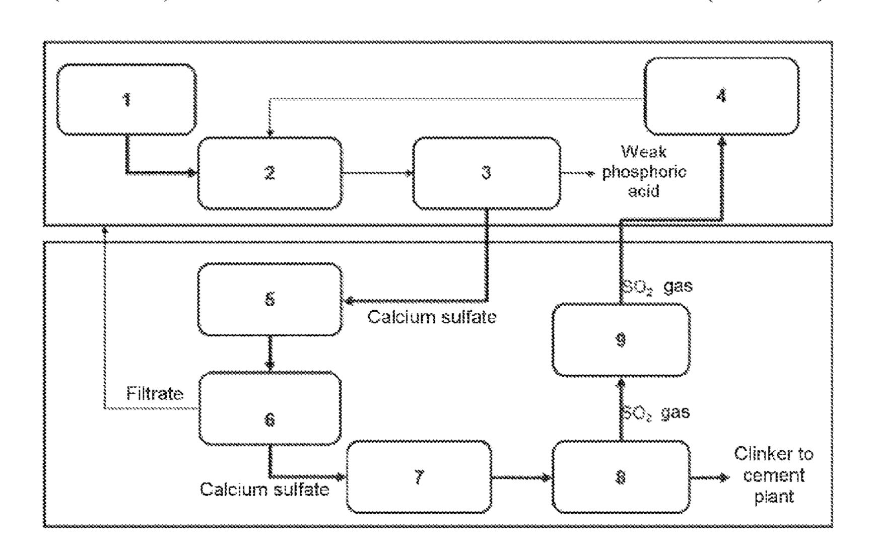
tures and reducing agents to obtain a raw meal mixture for cement clinker production, burning the raw meal mixture to obtain the cement clinker, with formation of sulfur dioxide as offgas, and subjecting the sulfur dioxide formed to offgas purification and feeding the sulfur dioxide as raw material to sulfuric acid production to produce the sulfuric acid. The sulfuric acid produced may be used as starting material in phosphoric acid production.
