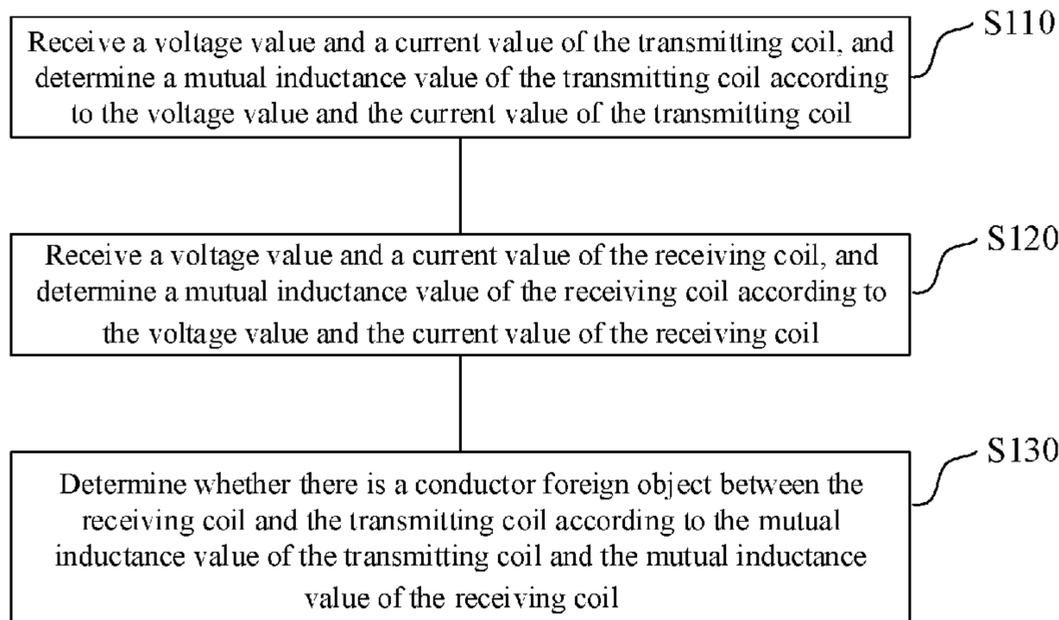
receiving coil; and determining whether there is a conductor foreign object between the receiving coil and the transmitting coil according to the mutual inductance value of the transmitting coil and the mutual inductance value of the receiving coil.
