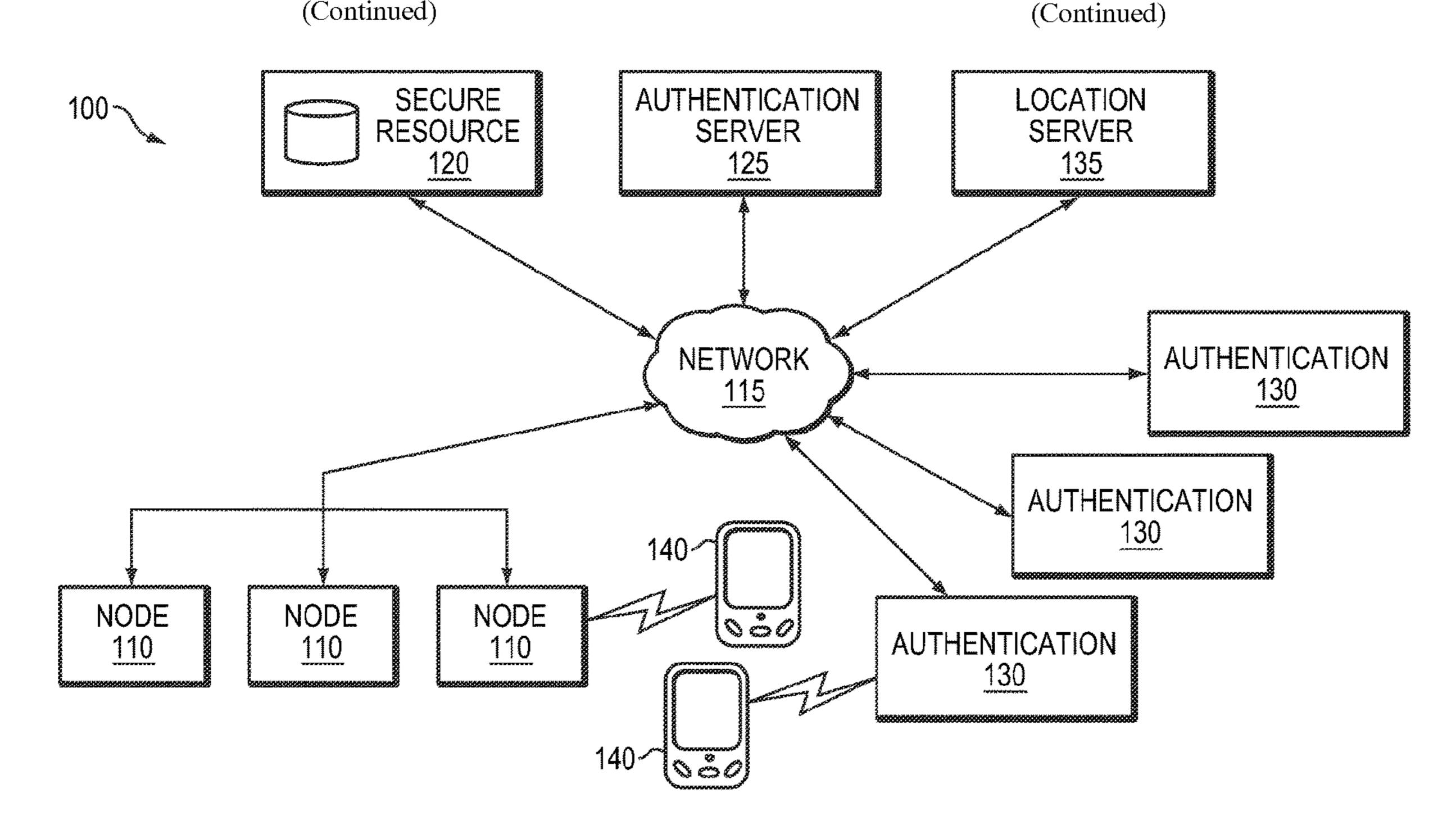
for locating the nearest such station and, in some embodiments, pair wirelessly with the station so that authentication thereon will accord a user access to the desired resource via a mobile device.
