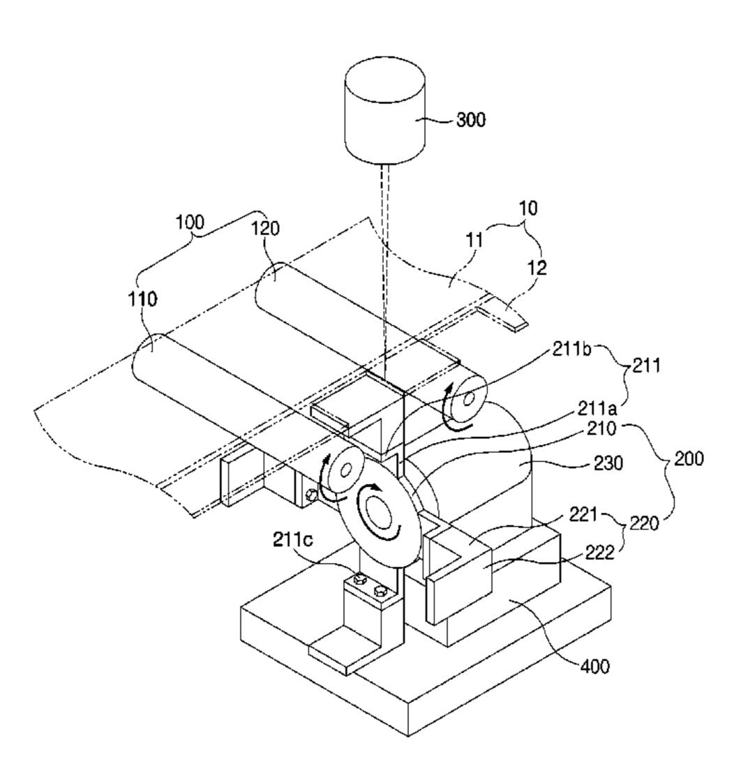
alternately support the non-coating portion disposed between the first and second transfer rollers when the rotation member is rotated.
