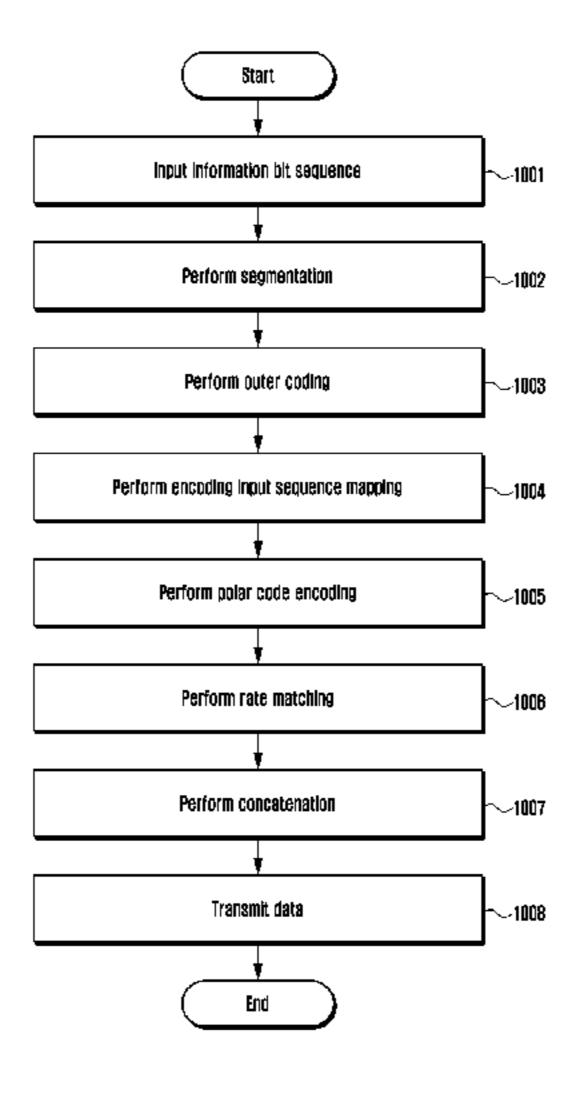
encoding the information bits according to the number of check bits, and transmitting the encoded information bits to a reception-end apparatus.
