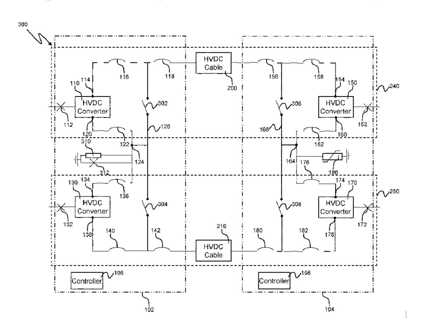
fourth HVDC converter (170) and the second transmission line (210); characterised in that: a neutral node (124) connecting the first HVDC converter (110) to the second HVDC converter (130) is coupled to a parallel combination of a resistance (310) and a neutral bus ground switch (312) for coupling the neutral node (124) to earth.
