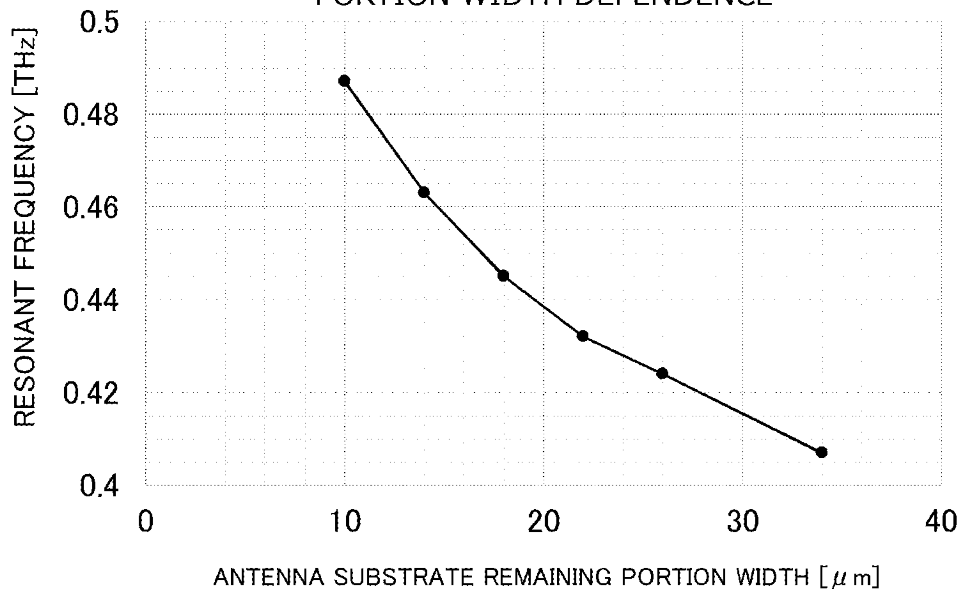
ANTENNA SUBSTRATE REMAINING-PORTION WIDTH DEPENDENCE
