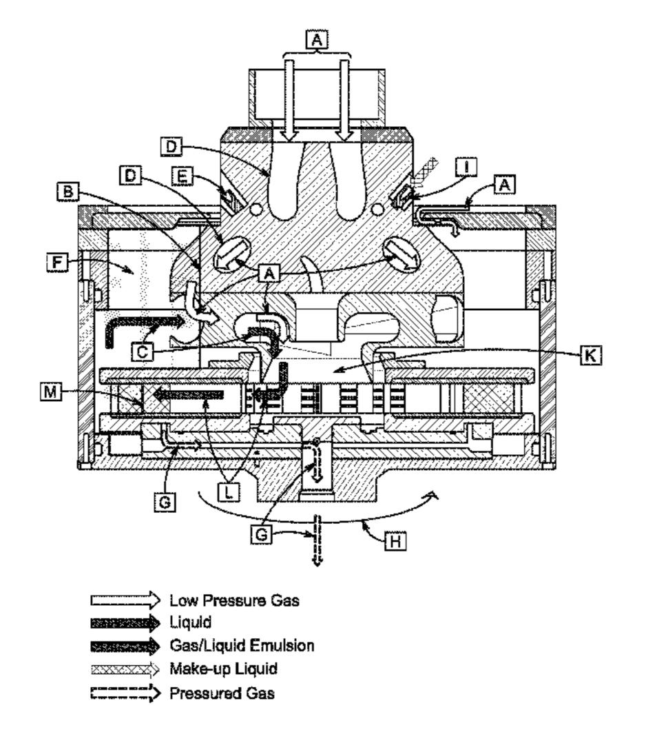
common pressure zone. Fluid is then forced into the compression channels where gas in the fluid is compressed as it travels from the common pressure zone toward the interior surface. The pressurized gas is separated from the liquid prior to leaving the compression channel assembly while the liquid is returned to the lake.
