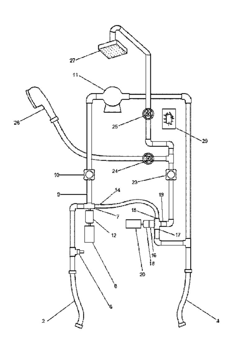
temperature preset in the device, wherein said device is composed of a housing, a temperature regulator, an LCD display, a LED ring, two water valves; a hot and cold water inlet; a three-way valve; a flowmeter connected to a pump; a thermostatic valve; a servomotor; and an integrated circuit board; and a method.
