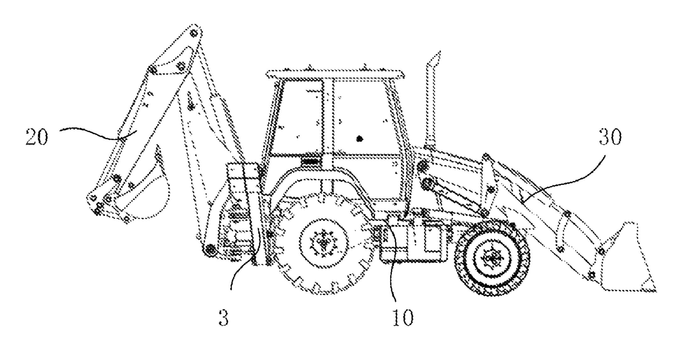
vehicle. The first stabilizer leg, the second stabilizer leg and the stabilizer foot cooperate to support the whole vehicle to improve the stability of the vehicle.
