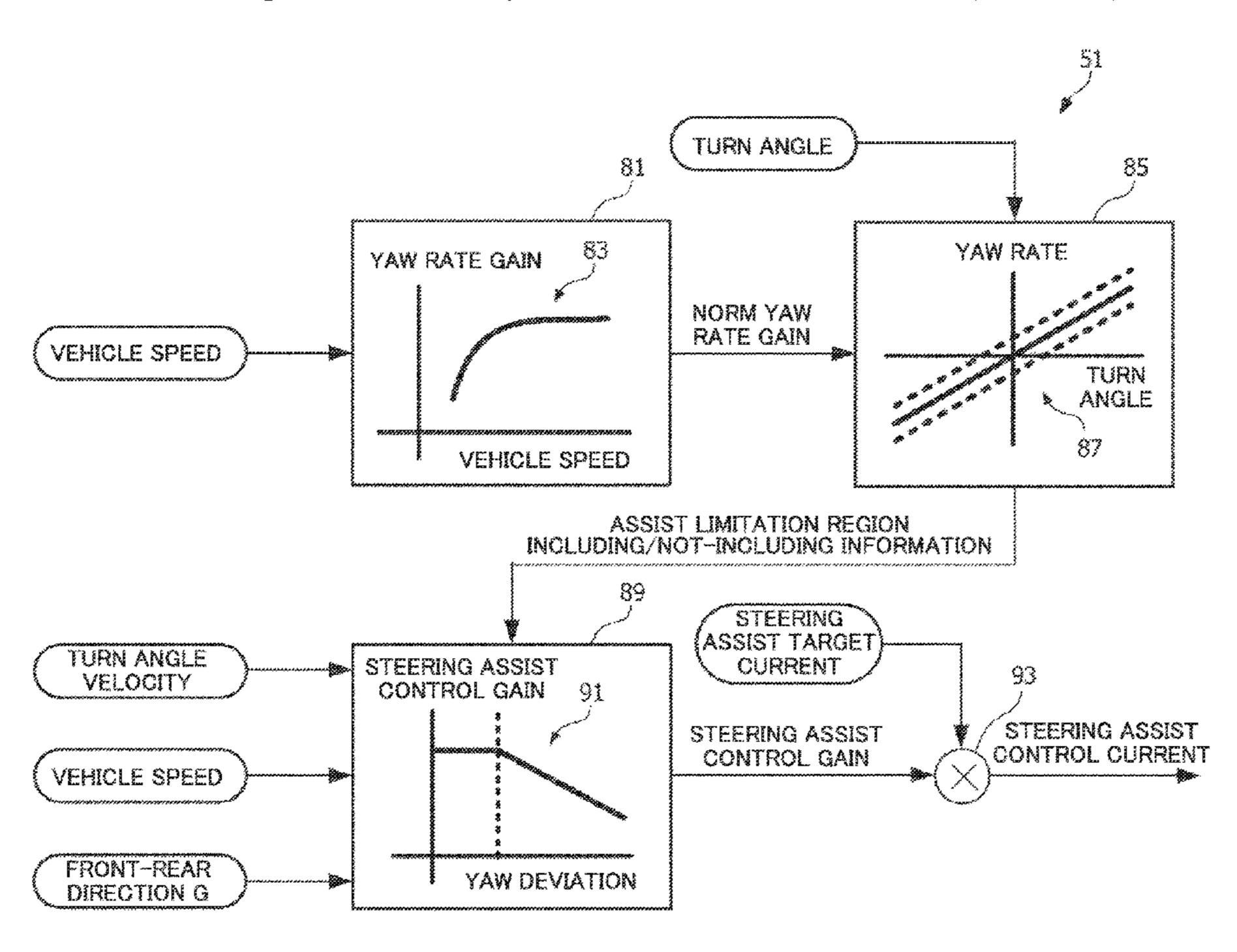
vehicle; and a steering assist control unit that performs steering assist control using the assist motor based on the information on the steering torque. The steering assist control unit performs the steering assist control based on the steering assist control amount set by the setting unit.
