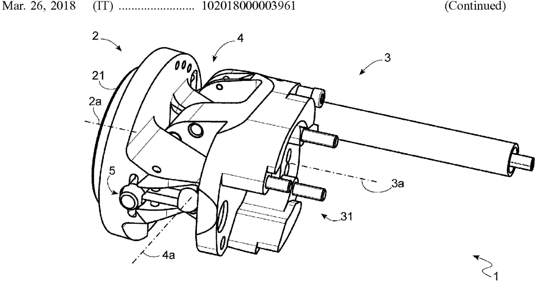
the bodies and around the axis of rotation, and elastic member placing the cable under tensile stress and working in opposition to the movement of the cable to define a rest position in which the cable and the elastic member exerts a zero resulting torque on the bodies and, and an activation position in which they exert a non-zero resulting torque on the bodies and, bringing the bodies and back to the rest position.
