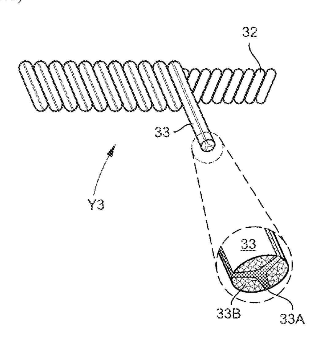
a repeating stitch pattern alternately zigzaging lengthwise up selected wales of the fabric structure and floating across the fabric structure in a widthwise course direction. The hybrid yarn cooperates with like knitted multi-wrapped hybrid yarns to form a continuous conductive matrix of static dissipative boxes in the fabric structure.
