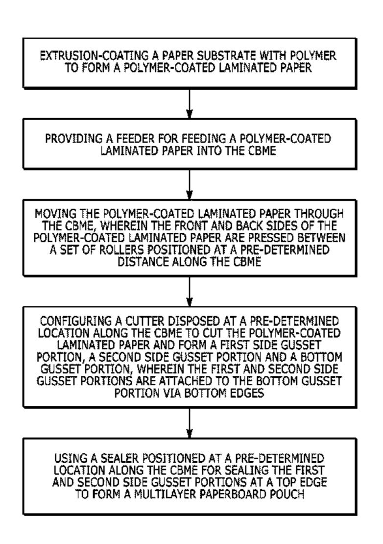
bottom gusset portion and the layers of the first and second gusset portions, respectively to form the finished multilayer paperboard pouch ready for sale and distribution to various retailers. It is to be noted that in the depicted embodiment various closure constructions and mechanism can be used for heat sealing the finished pouches.
