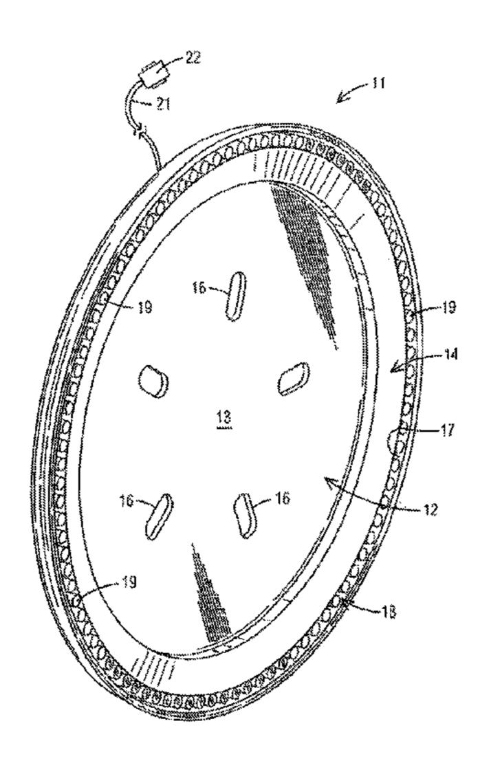
to be seen from behind as an indication that the vehicle is braking. A second portion of the ring of LEDs aligns behind the spokes and reflects off of the backs of the spokes to silhouette the rim against the glow of the reflected light.
