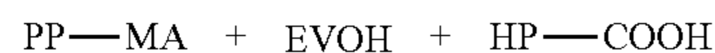
Scheme 4. A preferred multi-functional polyolefin structures (A) with EVOH as the coupling agent, prepared by the combination of PP-MA, EVOH, and HP reagent using reactive compounding process.
