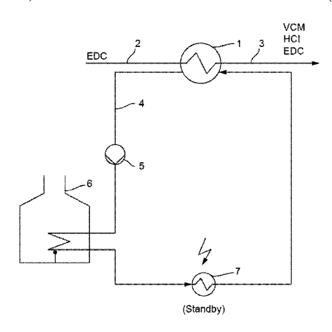
ing takes place and at least one first heating device by means of which heat is transported to the reaction medium in the reactor by means of the liquid or condensing heat transfer medium.
