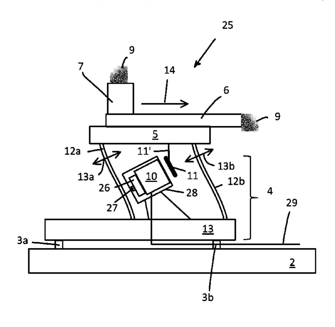
control may be used to also regulate the amplitude of the carrier arrangement and the associated mass flow m to a required value.
