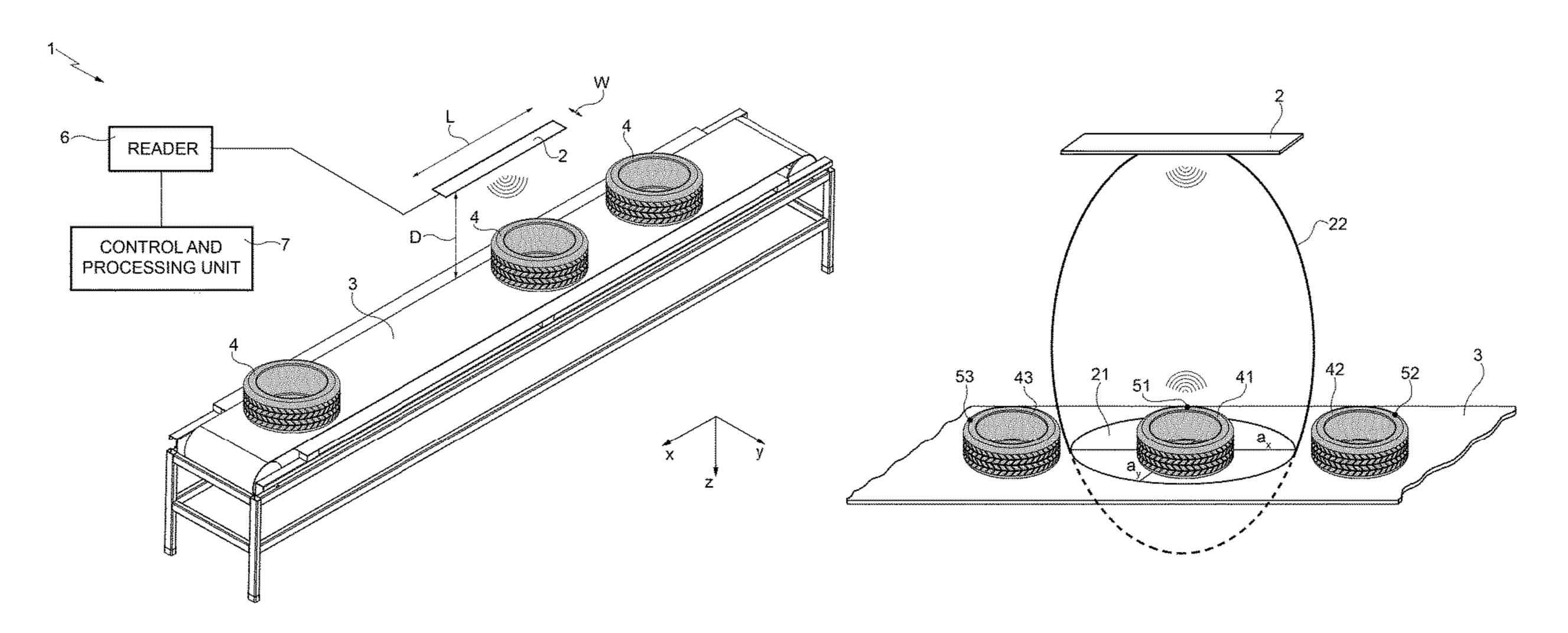
nary calibration step is applied to the reader and a reading and/or writing step is carried out by operating the calibrated reader.
