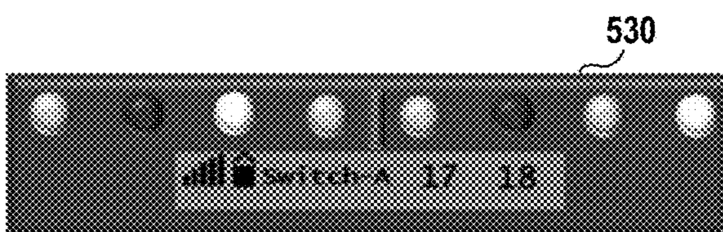
PLR for 2 ports with 4 lanes for each port, integrated status and activity LEDs, single LED row layout
