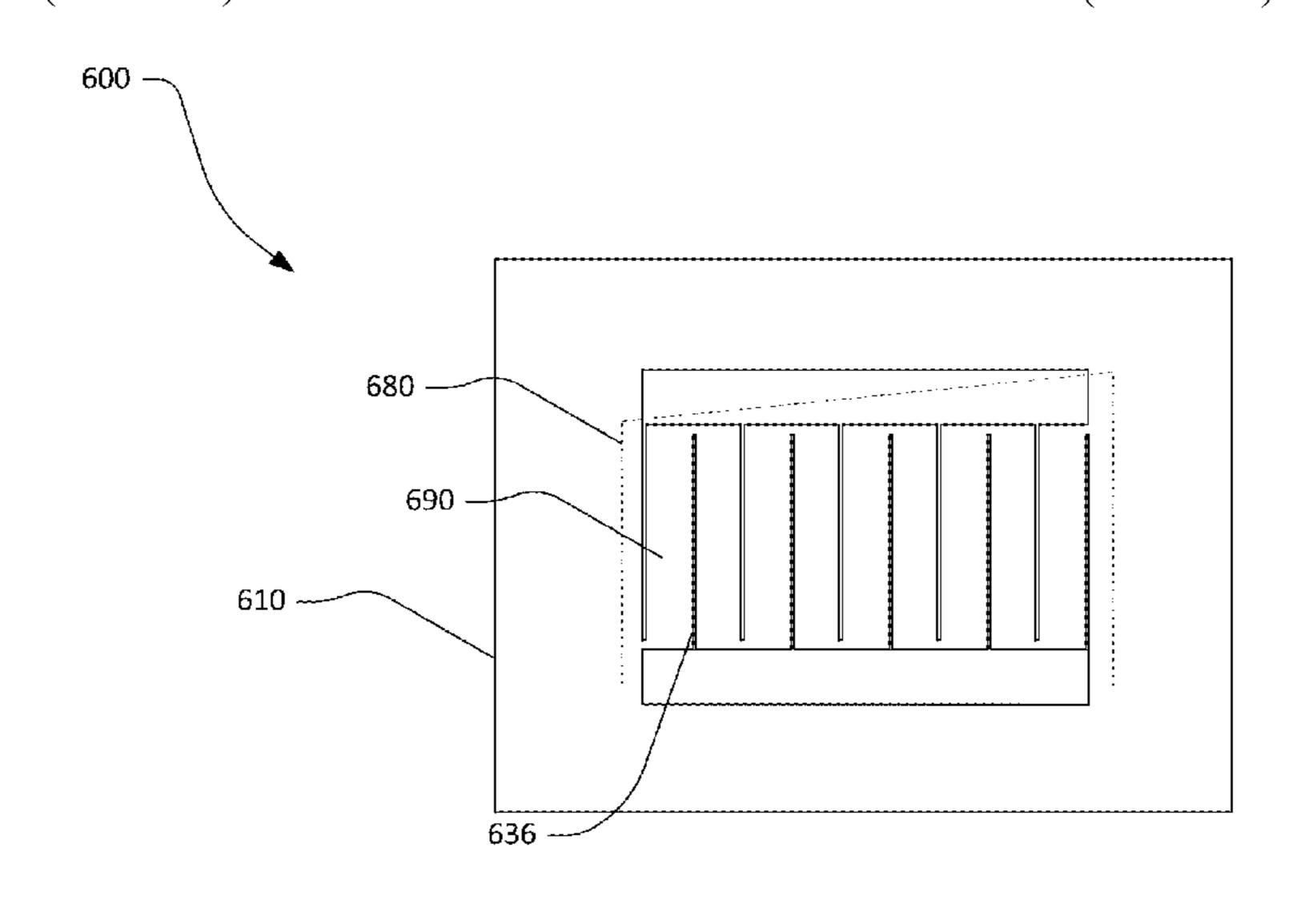
of an edge of the diaphragm is at an oblique angle to the fingers. The IDT includes a busbar disposed parallel to the edge of the diaphragm such that the interleaved fingers extend at the oblique angle from the busbar.
