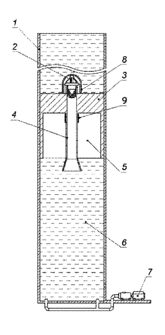
cross-sectional shape that follows the cross-sectional shape of the inner surface of the body. The means for preventing the platform from rotating can be embodied in the form of a protrusion on the platform, located in the corresponding recess on the inner surface of the body. The technical result of the claimed technical solution is manifested in an increased performance efficiency of the power generator.
