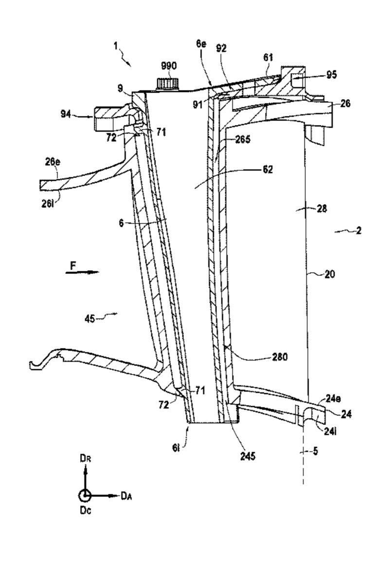
comprises at least one first radial shoulder projecting axially towards the inside of the blade, and each mast comprises at least one second shoulder projecting axially towards the outside of the mast configured to radially cooperate with a first shoulder and radially press the blade against the mast.
