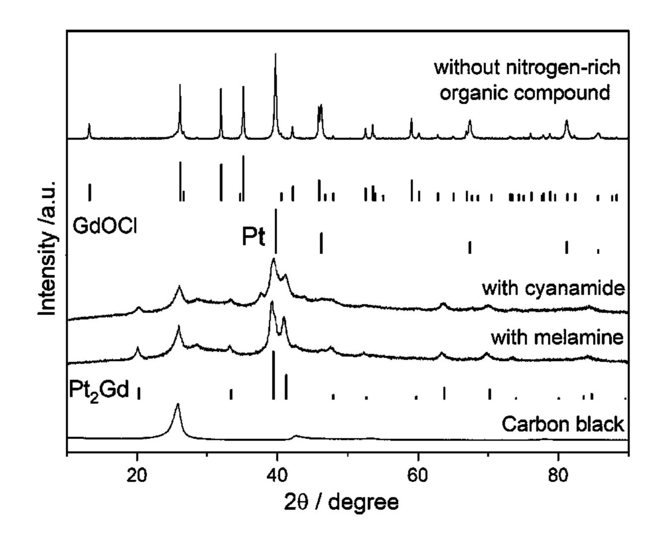
rich compound, and optionally a support material, to provide a precursor mixture, and heating said precursor mixture to a temperature of at least 400° C., in the presence of a gas comprising hydrogen (H<sub>2</sub>), to provide said alloy nanoparticles.
