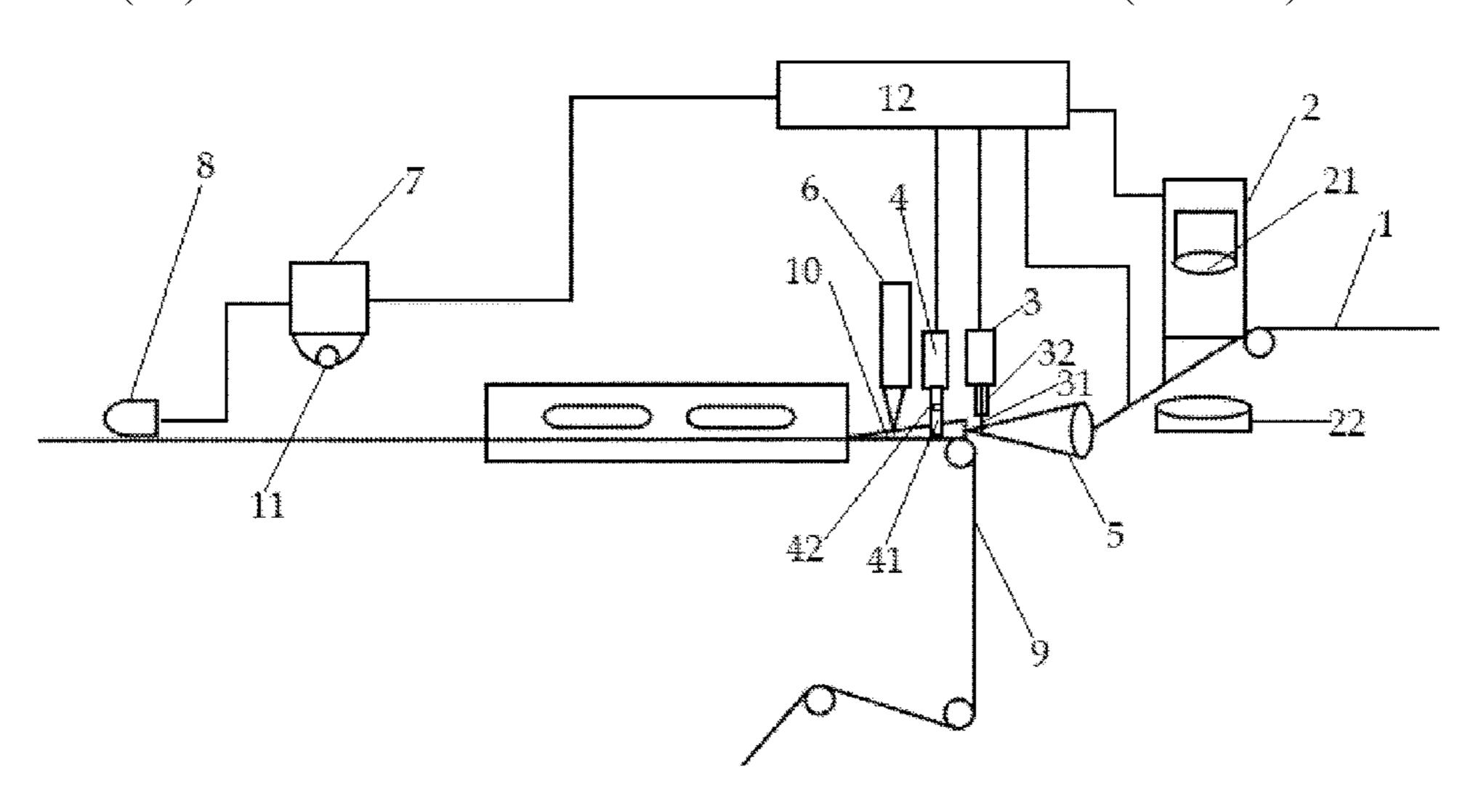
device and multi-flavor adding devices. According to shapes and types of flavors, the multi-flavor adding devices are arranged in different sections to obtain one-step formation of the multi-flavor composite structure filter rods. The present disclosure also discloses a one-step method of forming the multi-flavor composite structure filter rod using the one-step forming device.
