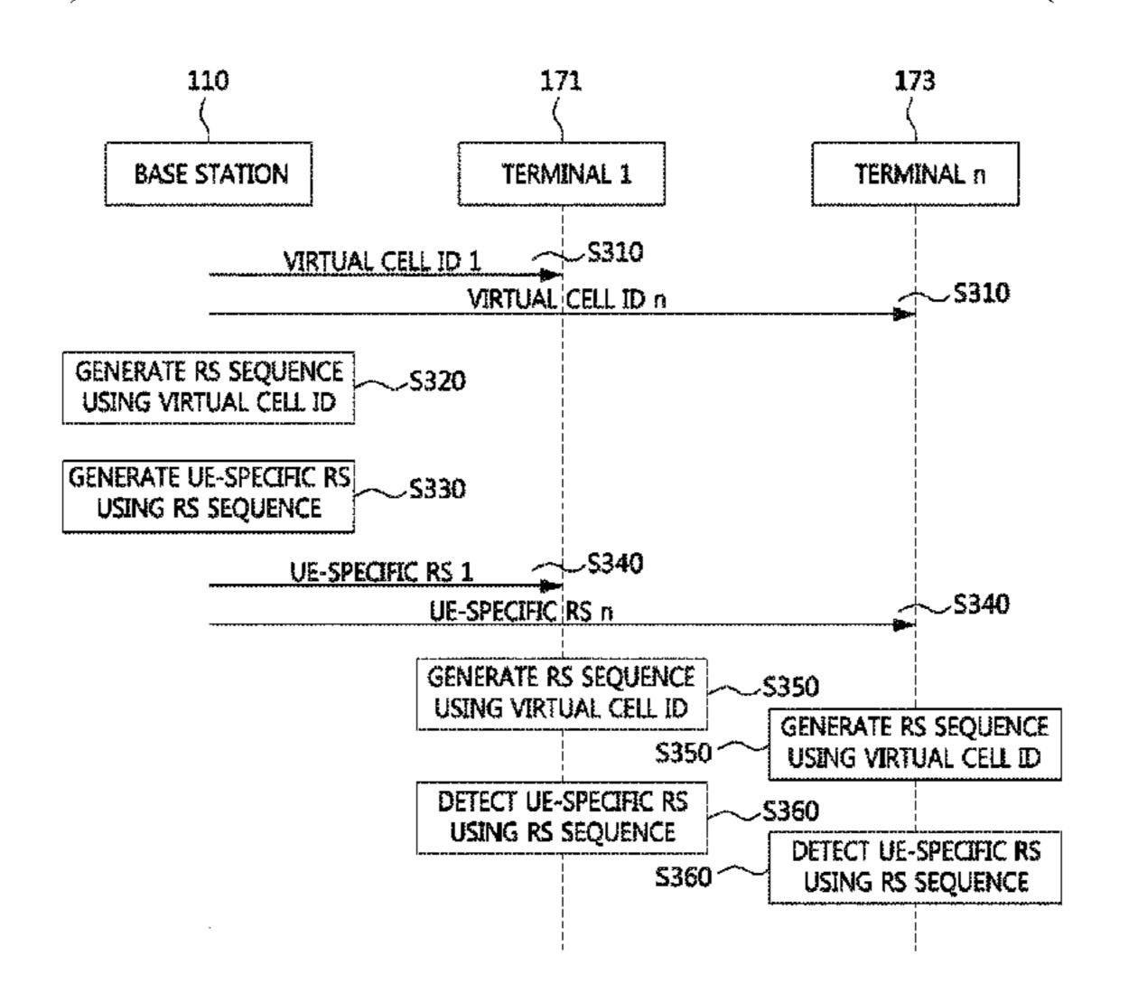
reception point has a wider transmission area than the at least one second transmission and reception point, and the first transmission and reception point and the at least one second transmission and reception point generate downlink transmission signals by using the same physical layer cell ID or virtual cell IDs allocated to each terminal, and then the terminals generate uplink transmission signals by using the allocated virtual cell IDs.
