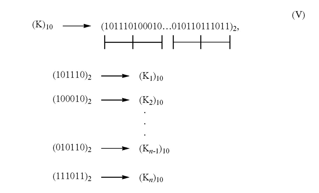
Establishing a chip sequence by means of a PN (Pseudo Noise) sequence generator according to any of the  $K_n$  keys that have been generated for the direct sequence spread spectrum (203),
