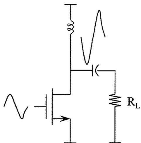
$$\text{Drain Efficiency} = \frac{P_{RF}}{P_{DC}} = \frac{V_{RFRMS} \times I_{RFRMS}}{I_{BIAS} \times V_{BIAS}} = \frac{\text{[Shaded Area]}}{8 \times \text{[Dashed Area]}}$$
