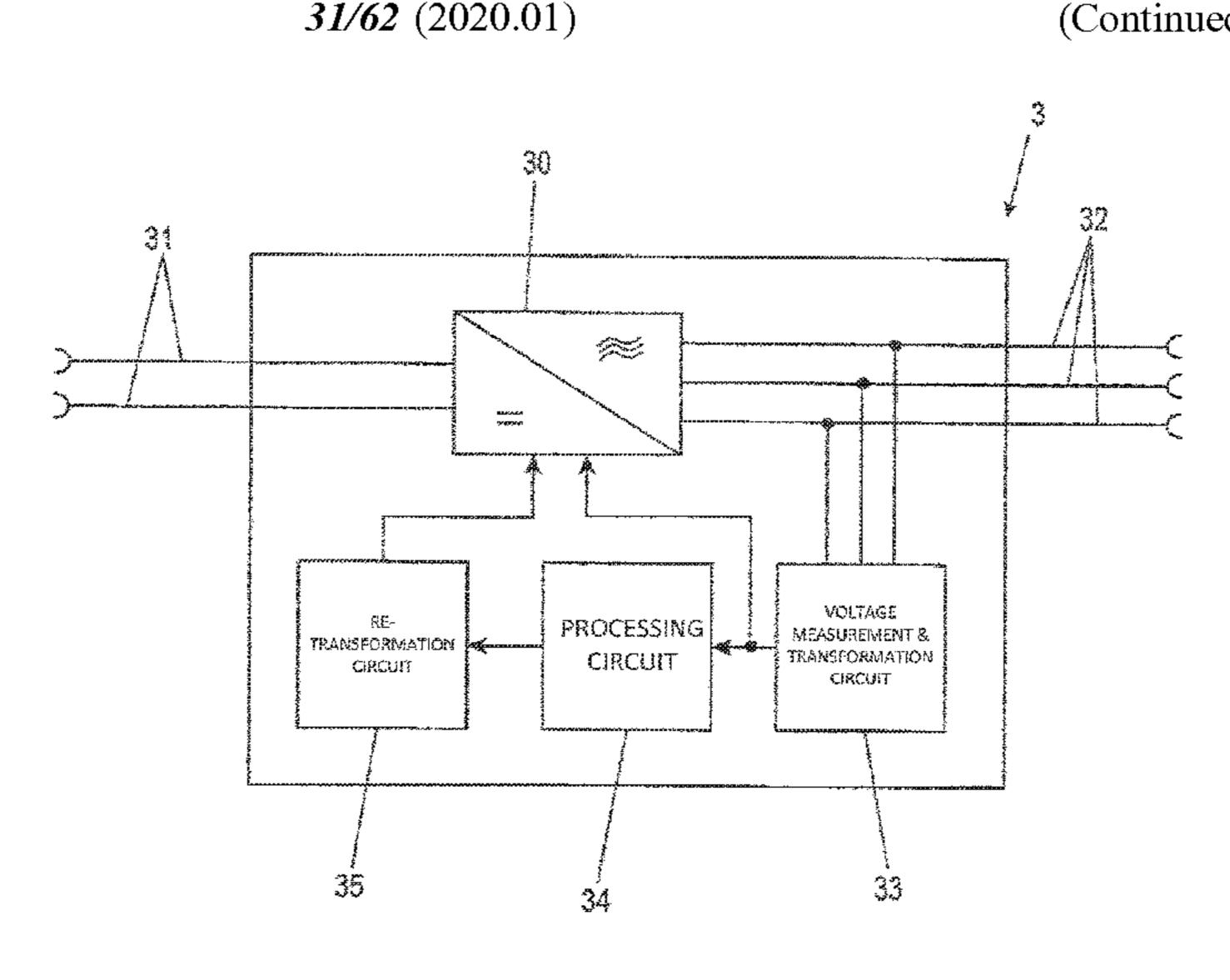
low-voltage side, determining estimated values of a zero phase sequence system voltage and of a phase angle of a zero phase sequence system at the high-voltage side from the measured delta voltages and phase voltages and phase angles at the low-voltage side, and transforming the positive, negative and zero phase sequence system voltages and the phase angles into phase voltages and/or delta voltages at the high-voltage side of the transformer.
