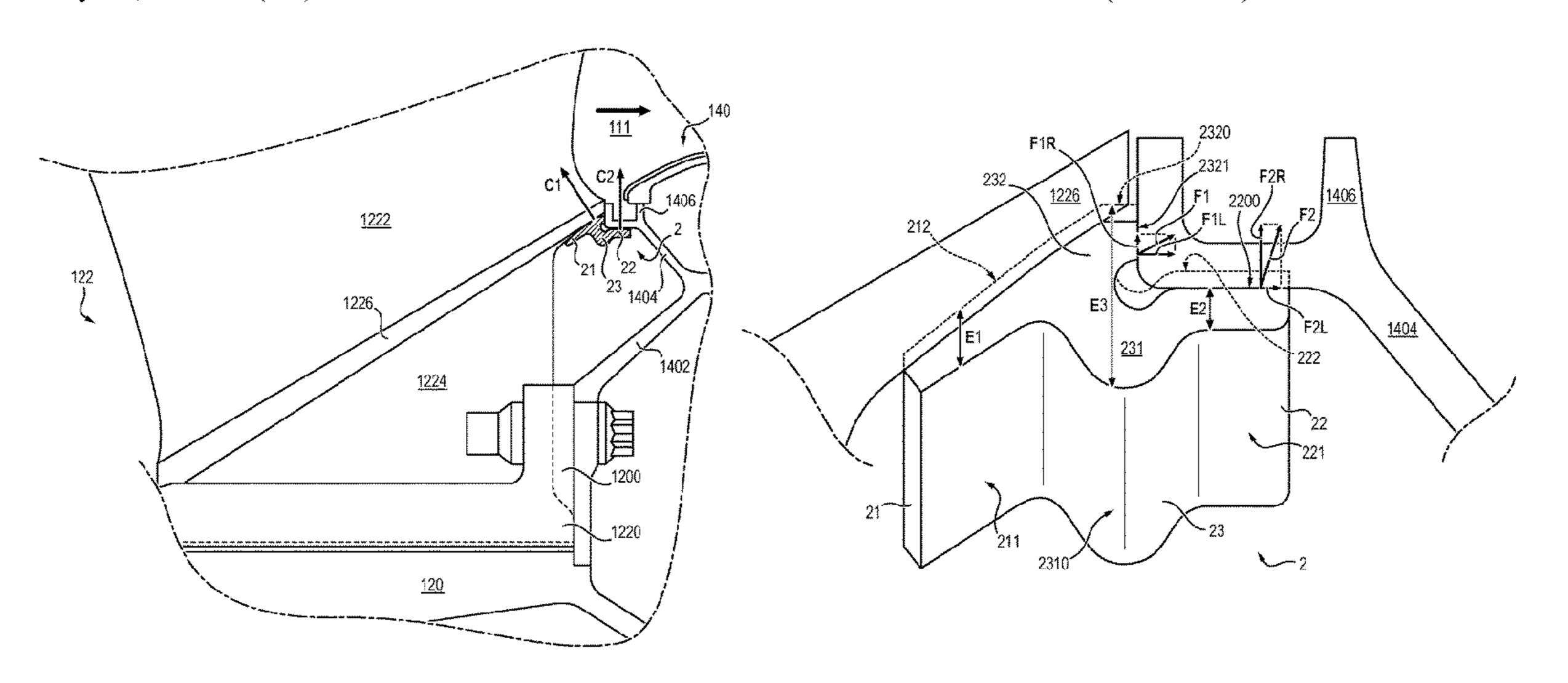
relative to the second rotor, the damper comprising: a first portion (21) bearing against the first rotor and having a first thickness, a second portion (22) bearing against the second rotor and having a second radial thickness, and a third portion (23) connecting the first portion (21) to the second portion (22) and having a third radial thickness, wherein the third radial thickness is greater than at least one of the first radial thickness and the second radial thickness.
