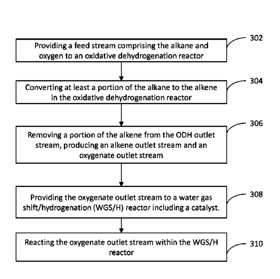
portion of the oxygenate and hydrogen are converted to an alcohol. Additionally, the alcohol may be dehydrated to form additional alkene and water.
