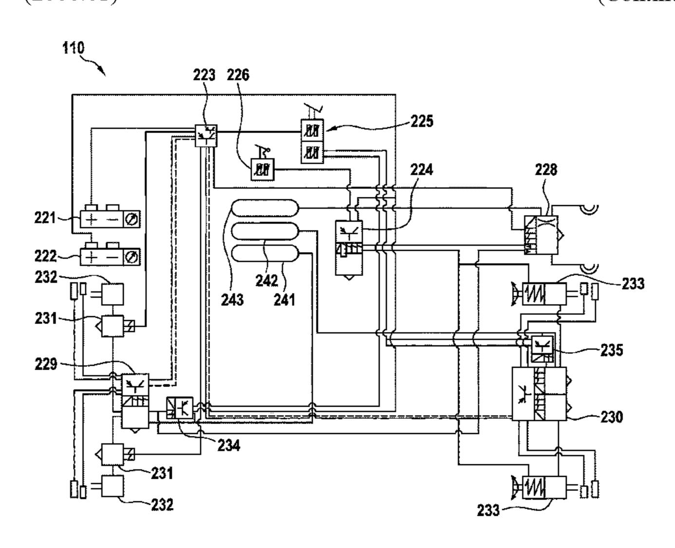
ond EPSU and redundant BPS. The first/second PMs are respectively fluidically connected to the first/second APMs. The redundant-BPS issues a first control-signal (CS) for the EBCU and a second CS for controlling the first/second PMs. The first PM commands pneumatic-control-pressure for the first APM depending on the second CS from the redundant-BPS. The second PM commands pneumatic-control-pressure for the second APM depending on the second CS from the redundant-BPS.
